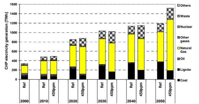
Figure 8: Net electricity generation of CHP plants in the EU27 by energy carriers in different cases
