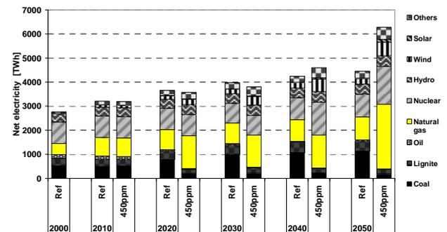
Figure 6: Net electricity generation in the EU27 by energy carriers in different cases
