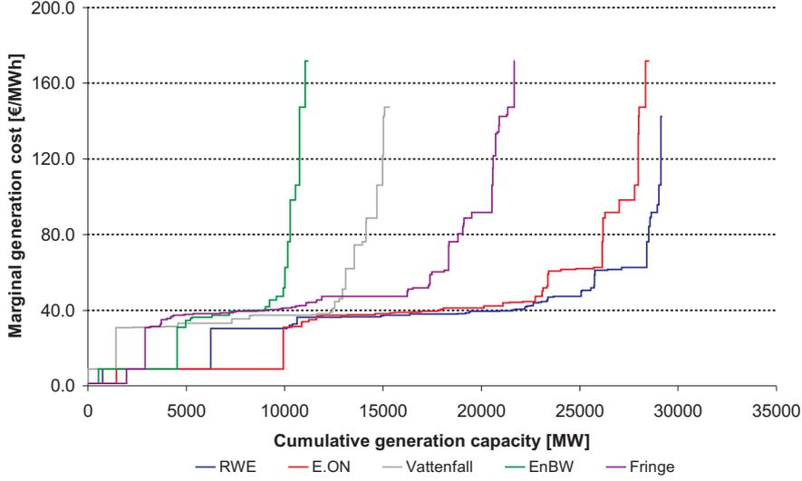
Fig. 4. Merit Order curves of generators and competitive fringe in Germany
