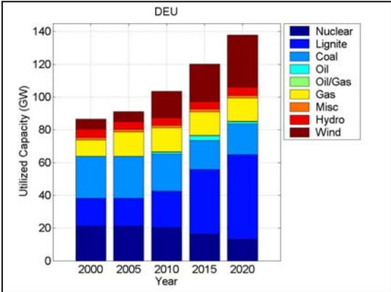
Figure 7 Utilized capacities in the stochastic BAU scenario.
